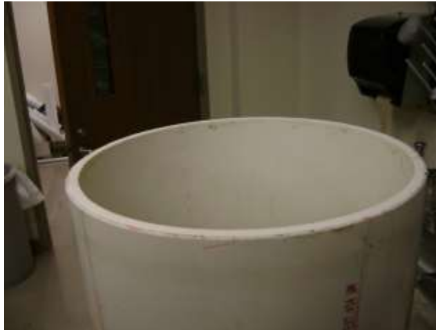
Figure 1 - End of Casing after smoothing
