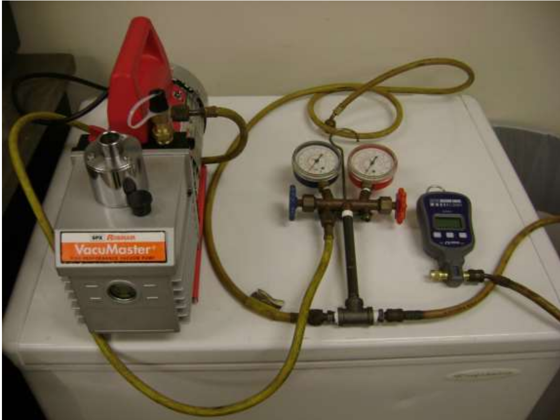
Figure 4 - Pump, Manifold, and Omega Gauge connected on top of freezer
